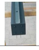
1A - setting the posts in the ground: Set the aluminum postanchor with about 75 cm buried in the ground. Use a rubber or wooden hammer, or cover the head of the postanchor to avoid damaging. Level the postanchor. Remove, if necessary, some ground for proper alignment later on, especially important if you use 200 cm posts.
