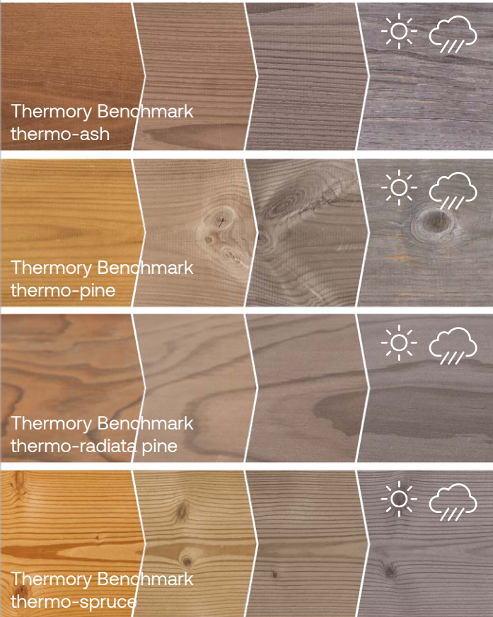
After installation Unooled wood exposed to UV light
